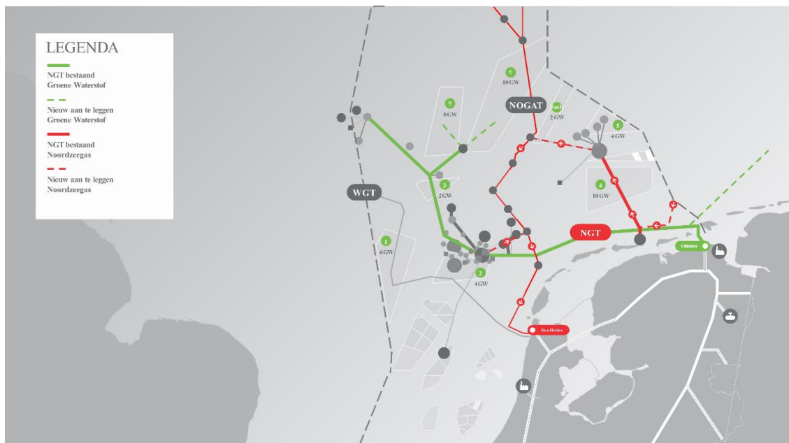
Possible scenario for potential new pipelines (dashed red) to re-route gas from NGT (green) to NOGAT (red through).
